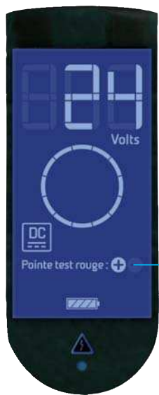
Example of continued 24 V detection, display is BLUE because < 50 V.
